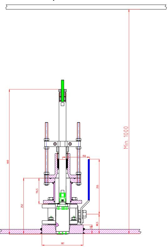
The Sea Valve should be placed in a service accessible place, large enough for installation and disassembly of the sensor unit.
